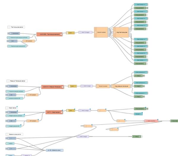
Node-Red, a flow based programming language, was used to connect all the sensors together with the state machine. To the left is an overall flow diagram for the alle the sensors, valves, and including the state machine.
